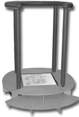
Fig.5. Synapsys Posturography System with implemented force platform used for S.O.T test
