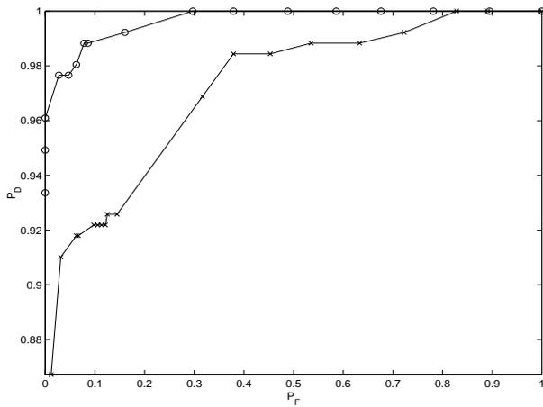
Figure 6: ROCs for the EMD-based detector 'o' and that of the DWT-based detector 'x'.
