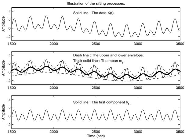
Figure 2: Illustration of the sifting process.
