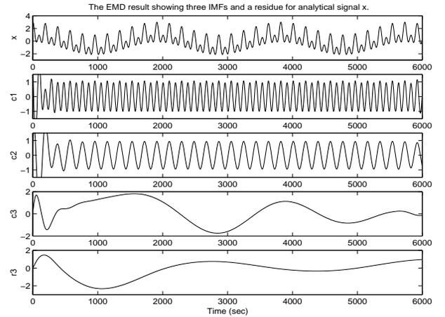
Figure 4: The EMD result showing three IMFs and a residue for analytical signal  $x$ .
