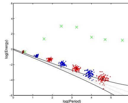
Figure 3 – Log-log diagram of the energy and dominant period of the different intrinsic modes identified by the EMD technique. The separation between observations (green crosses) and Monte-Carlo simulations of red-noise (red and blue dots) displayed in this figure indicate that a range of atmospheric waves can be observed in the Scott Base MF radar data. The full and dotted lines indicate the theoretical bounds (99 % and 75% limits) within which white-noise should fall.
