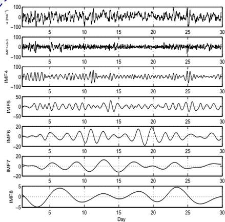
Figure 1 – The results of application of the EMD technique to the zonal wind time series observed by the Scott Base radar at 90 km in January 2006 are displayed. The upper panel in this figure displays the original time series. The second panel contains the summation of the first to third IMFs, the third panel contains the fourth IMF, the fourth panel the fifth IMF etc.
