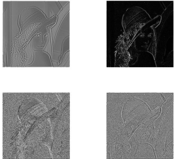
**Figure 5. left-up: 1st IMF, right-up: amplitude, left-down: phase orientation, right-down: phase angle.**
