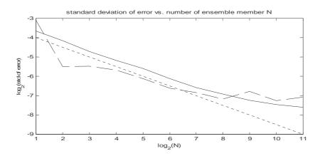
**Figure 5:** The standard deviation of error as a function of the number of ensemble members. The solid line is for the high frequency intermittent signals, and the dashed line is for the low frequency fundamental signals. The dotted line is the theoretical line predicted by Eq. (6) with arbitrary vertical location, used as a reference.
