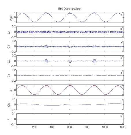
**Figure 4:** The IMF-like components of the decomposition of the original input in Figure 1a using the EEMD. In the EEMD, an ensemble member of 50 is used, and the added white noise in each ensemble member has a standard deviation of 0.1. In panel a, the mean of the noise modified input is plotted. In panel 5, the original input (red line) is also displayed for comparison.
