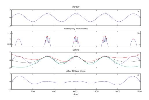
Figure 1: The very first sifting process. Panel a is the input; panel b identifies local maxima (red dots); panel c plots the upper envelope (red) and low envelope (blue) and their mean (black); and panel d is the difference between the input and the mean of the envelopes.
