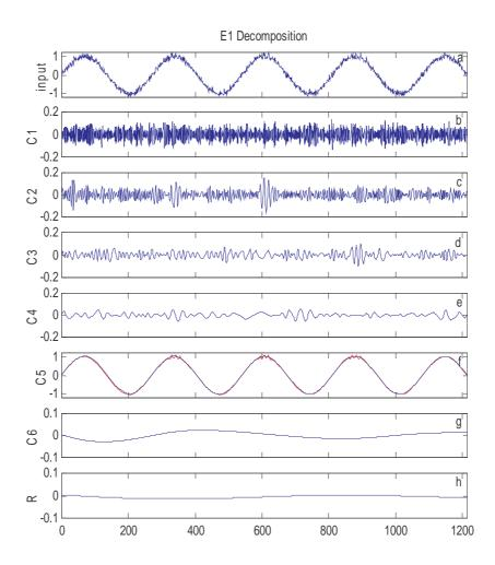
**Figure 3:** The intrinsic mode functions (panels b-g), and the trend of the modified input (panel a). In panel f, the original input is plotted in red as a comparison.
